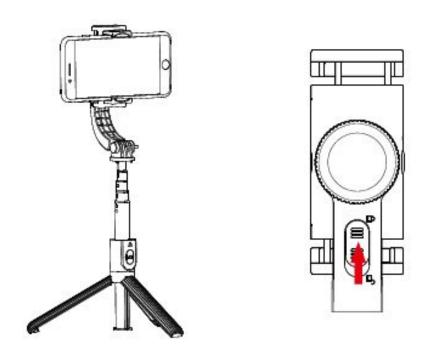
When the battery of the pan-tilt is low, the red light will flash to remind you to recharge it. You can do it by using your microUSB cable and charging the selfie stick. Once the charging process starts, the red light will stay on until the selfie stick is fully charged.
